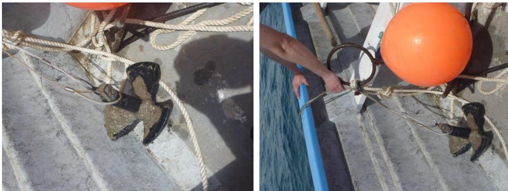
Figure 2. Detail of river anchor, wires and lock used to construct the moorings to deploy acoustic detectors in the buoys delimiting the Protection Refuge for Vaquita. After one month of soaking it do not appears any trace of stain or damage.
